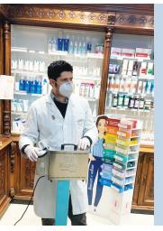
The automated disinfection system Bugsby evaporates a disinfection liquid with the help of a pump, which sucks the liquid into the system, and a heat exchanger, which heats the liquid until it evaporates in the surrounding air. The system can be operated by an electronic control panel.
